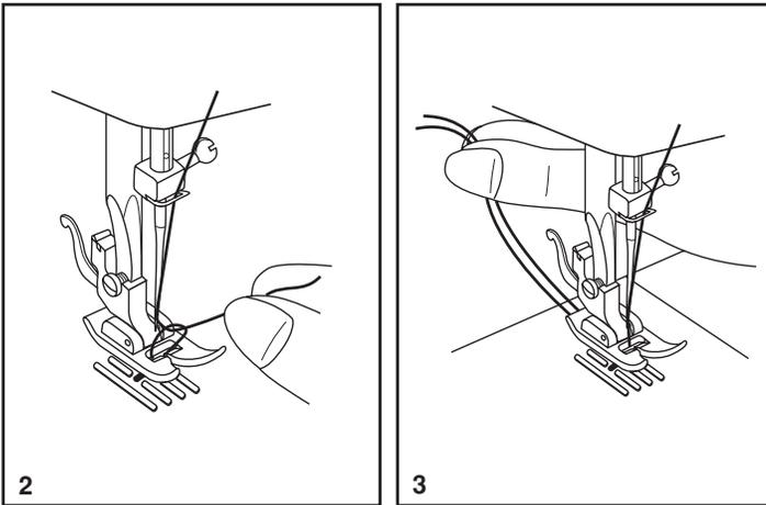
Gently pull on the upper thread to bring the bobbin thread up through the needle plate hole (2). Lay both threads to the back under the presser foot. (3)
